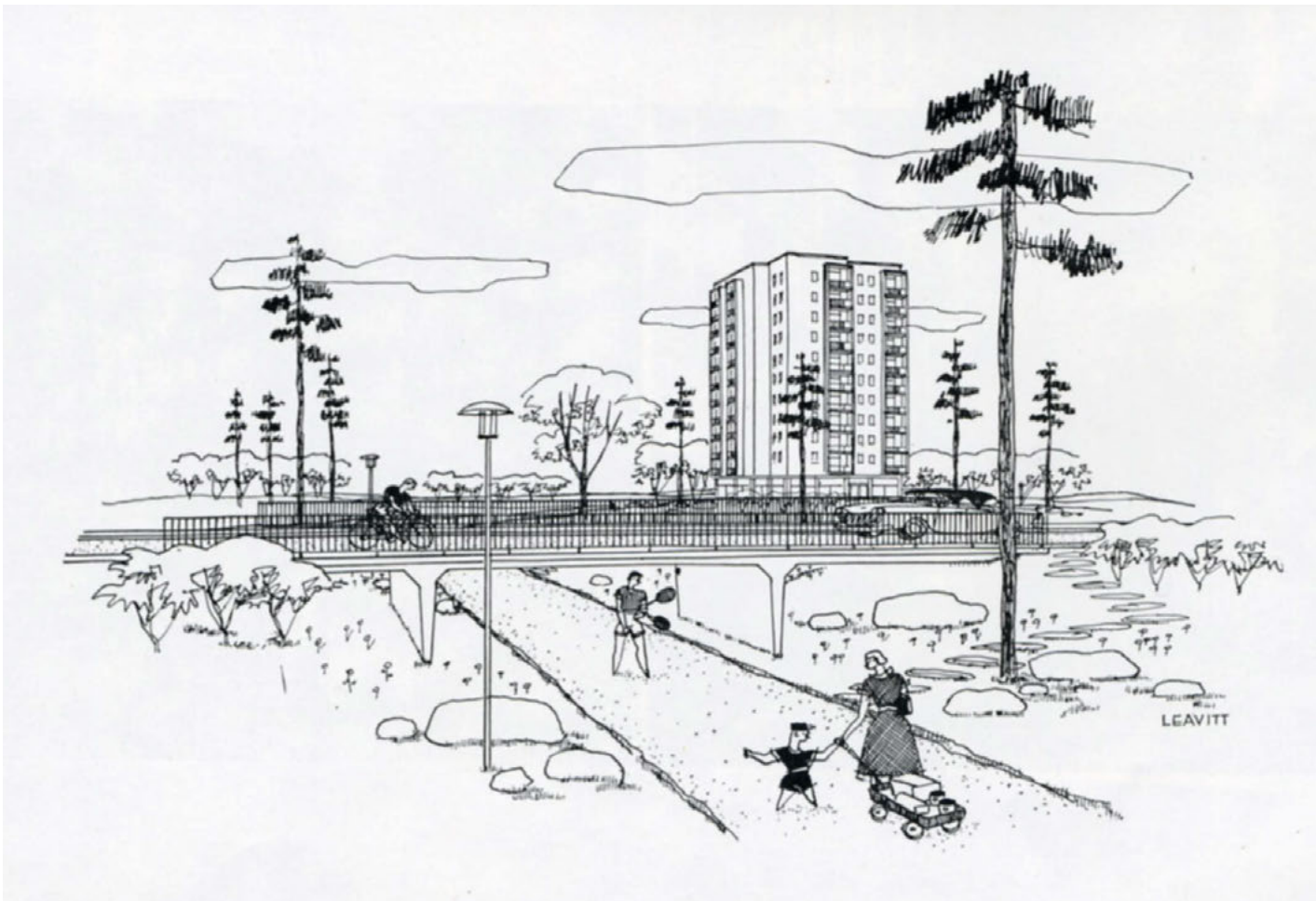
Sketch showing Vällingby's traffic separation, inspired by Clarence S. Stein's Radburn. Kidder Smith, G. E.: Sweden Builds , New York: Albert Bonnier, 1950/57.
